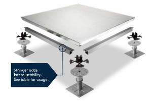
The pedestals are of a Zinc plated steel construction, ensuring electrical continuity, pre-assembled to help minimize installation time. The pedestals have a locking nut to ensure that once adjusted and locked there is no movement in the pedestal head.
